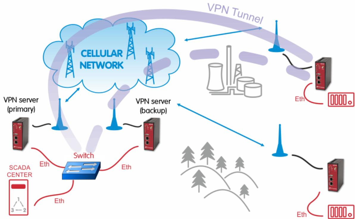
This solution increases the hardware reliability of the center. A redundant VPN concentrator (cluster) solution may be used to further improve the reliability. However a leased line to the Cellular network operator center is more reliable solution and it is recommended whenever the reliability of the network really matters.
