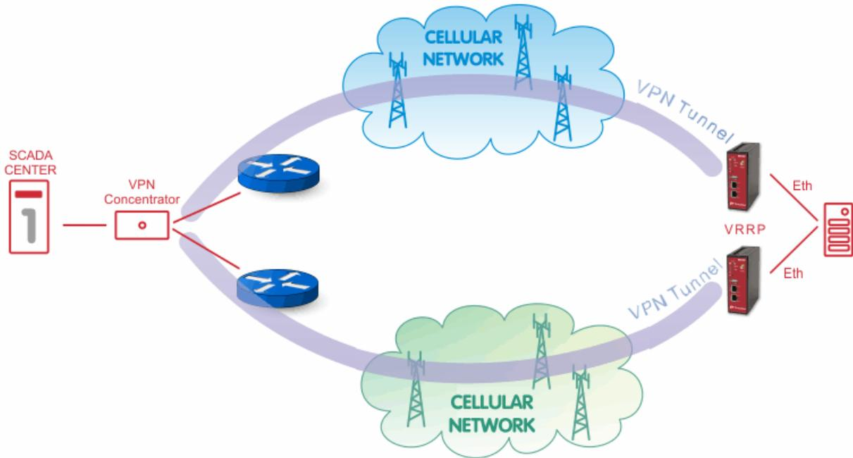
A fully redundant solution for both the center and remote locations is certainly possible:
