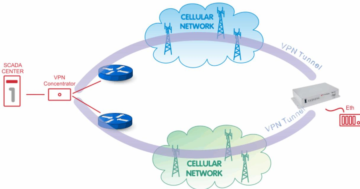
The fully redundant solution of the center is possible as follows:
