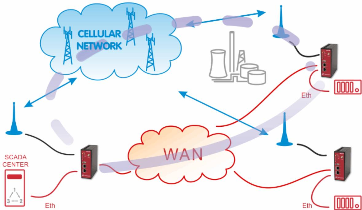
Under usual circumstances, VPN tunnels between remote and central M!DGE/MG102i units are established over the WAN network. When the WAN fails, the traffic from/to the respective remote M!DGE/MG102i is automatically redirected to the cellular network.
