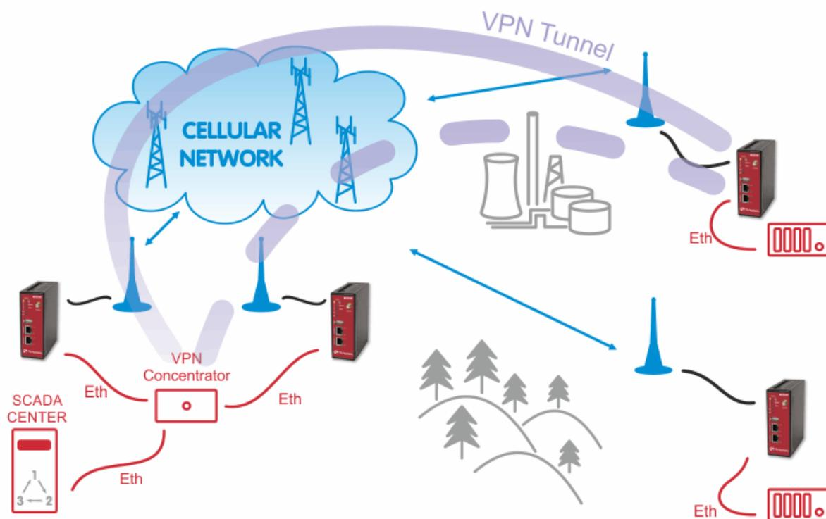
Two M!DGE/MG102i units with Virtual Router Redundancy Protocol (VRRP) functionality can be used. The VRRP creates one virtual IP address for both units and this IP address is active for the local LAN. Two independent SIM cards (one in each unit) are used for obtaining public mobile IP addresses. The OpenVPN tunnel is the recommended tunnel type.
