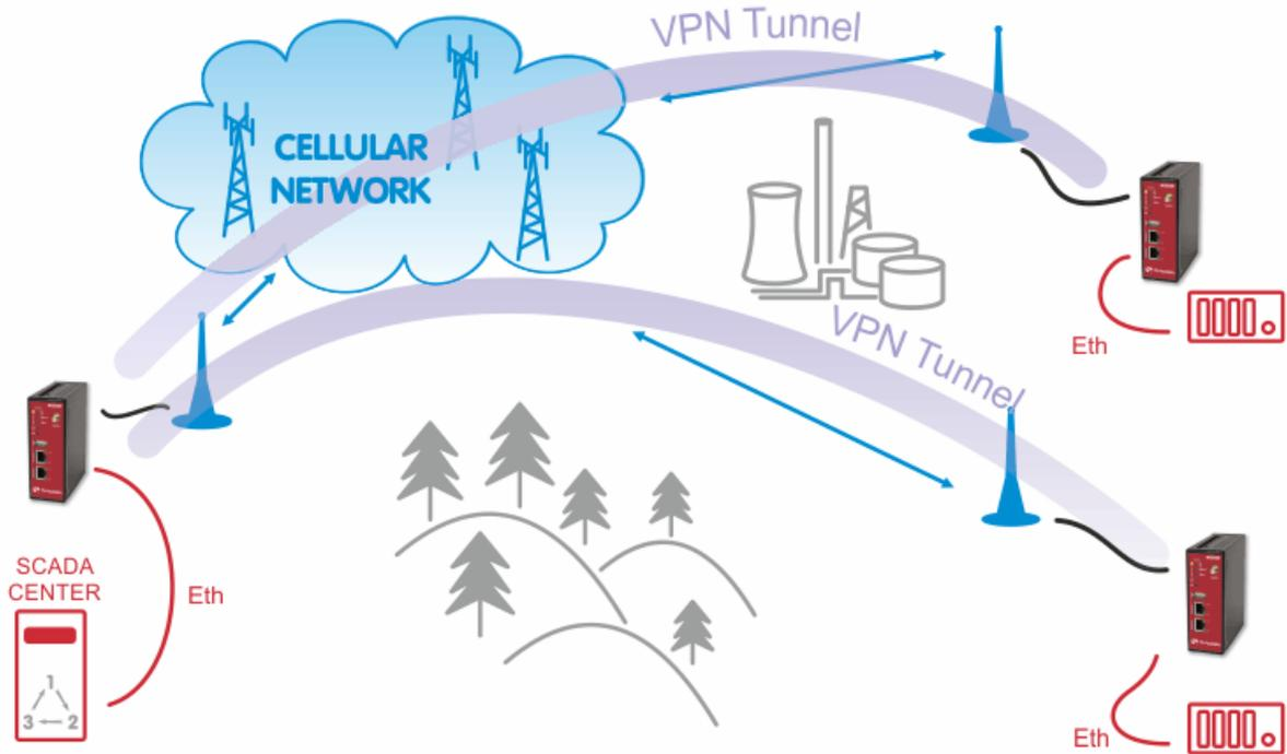
The central unit must be reachable from all clients. The central unit must have the public IP address which can either be static or dynamic. In case of dynamic IP address, the dynamic DNS functionality has to be configured and enabled.
