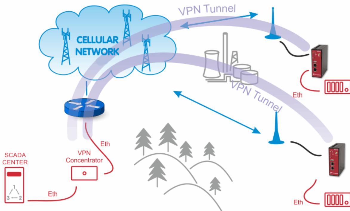
When a higher number of tunnels (i.e. a higher number of remote units) is required, VPN concentrator has to be used – a special router (e.g. CISCO) for IPsec tunnels or an ordinary PC (Linux/Windows) for OpenVPN tunnels.
