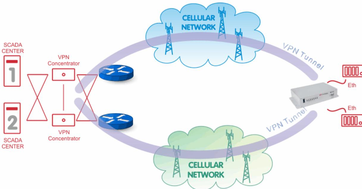
Remote redundancy with two MIDGE/MG102i units with VRRP activated – this solution can handle both the network service failure and the MIDGE/MG102i router (+ antenna installation) HW fault:
