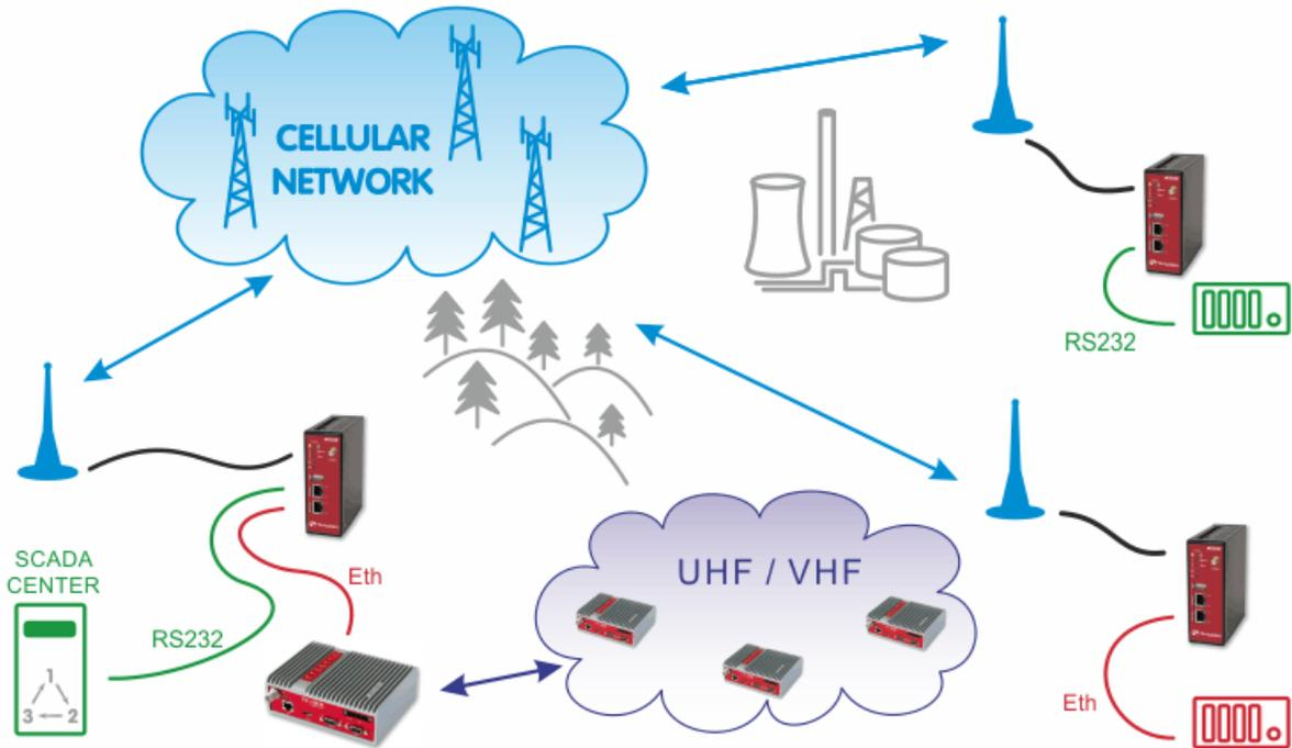
The picture above describes an arrangement, where part of the remote sites is connected over a private UHF/VHF radio network (e.g. sites requiring 99.9% availability) and the remaining sites are connected over the cellular public network (e.g. distant, isolated locations where it would be uneconomical to extend the radio coverage to).
