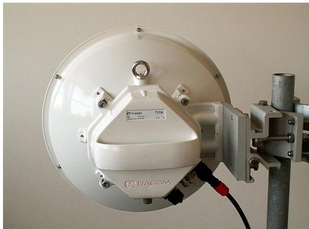
Fig. 5.1: Left-side mounting – horizontal polarization
