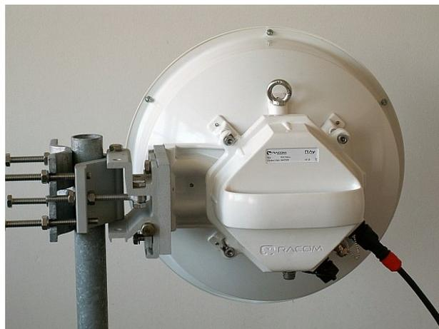
Fig. 5.3: Right-side mounting – horizontal polarization
