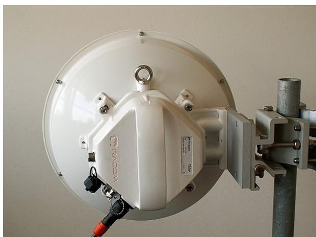
Fig. 5.2: Left-side mounting – vertical polarization
