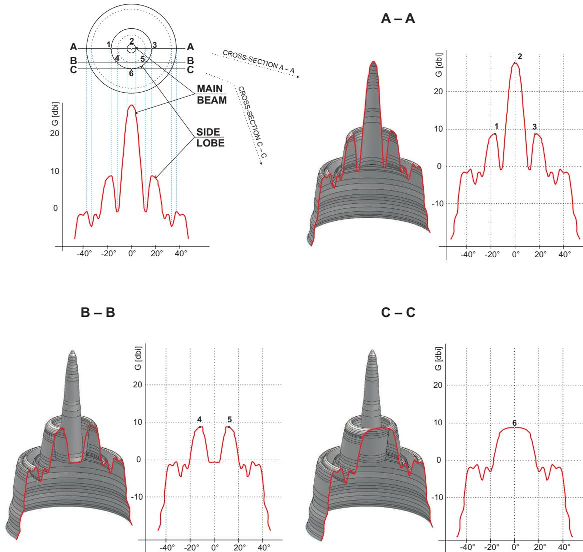
Fig. 5.70: Radiation diagrams
