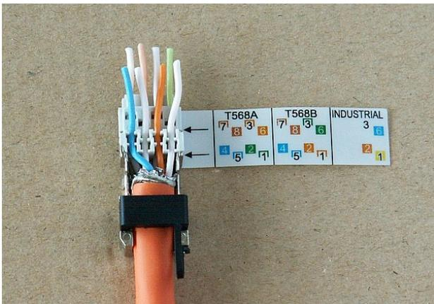
Fig. 5.54: All conductors in the connector
