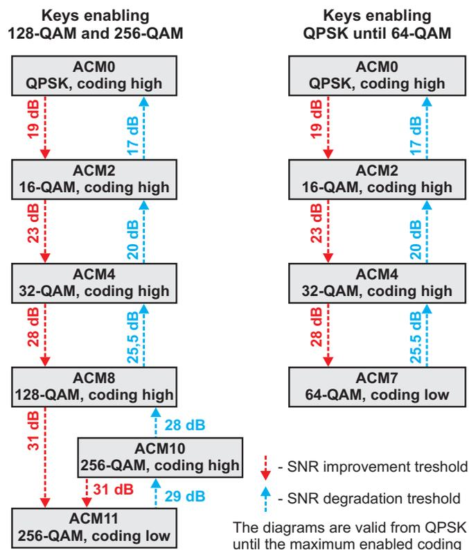
Fig. 9.1: Status diagram of ACM switching according to SNR state
