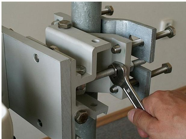
Fig. 5.16: Horizontal adjustment of the antenna direction
