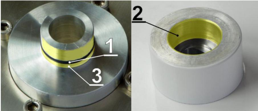
Fig. 5.26: Grease points on the antenna pivot and FOD unit bush
