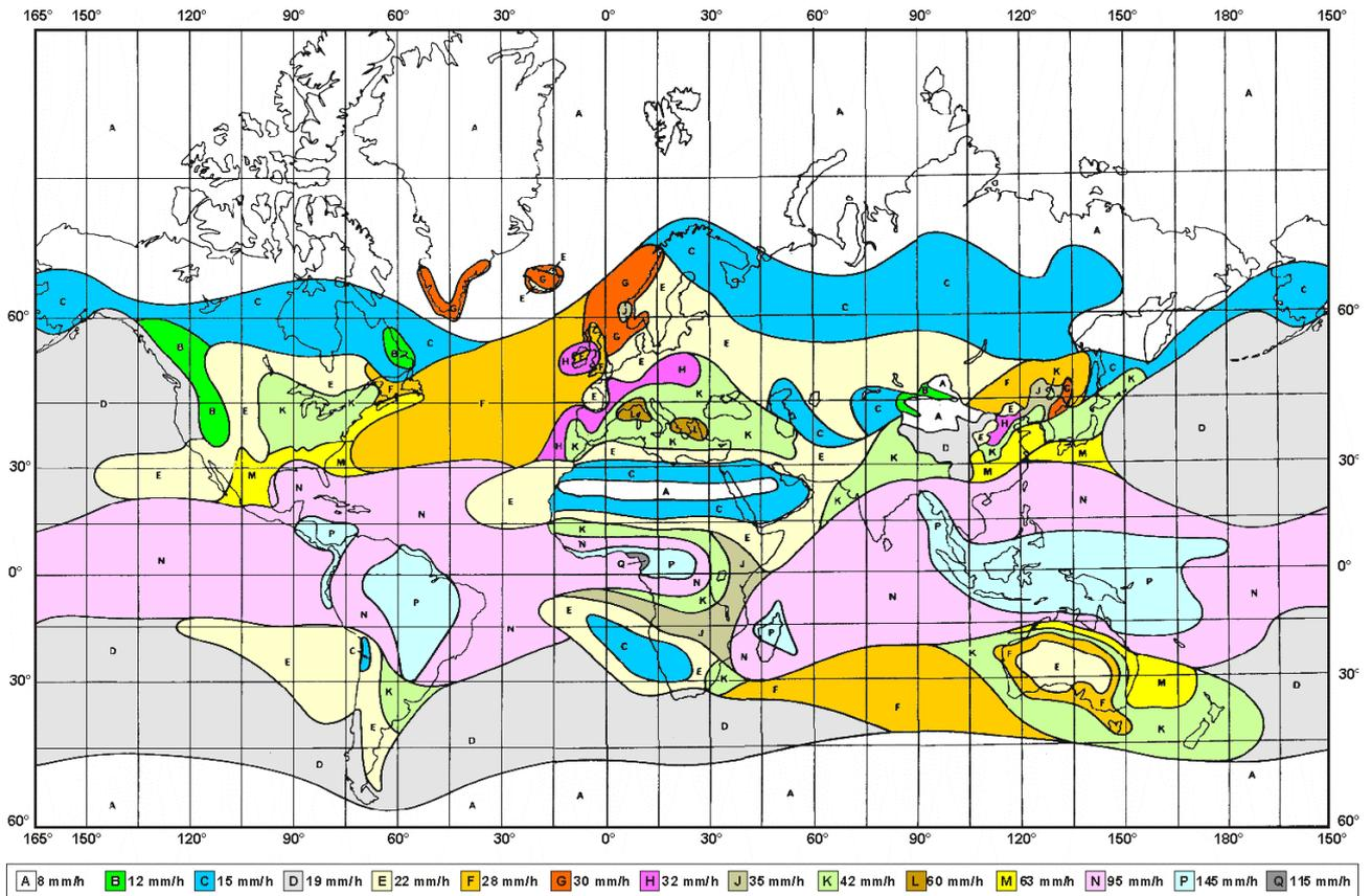
Fig. 2.1: Rain zone map, based on Rec.ITU-R PN.837-1
