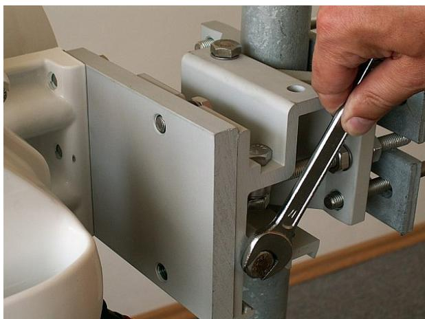
Fig. 5.17: Vertical adjustment of the antenna direction
