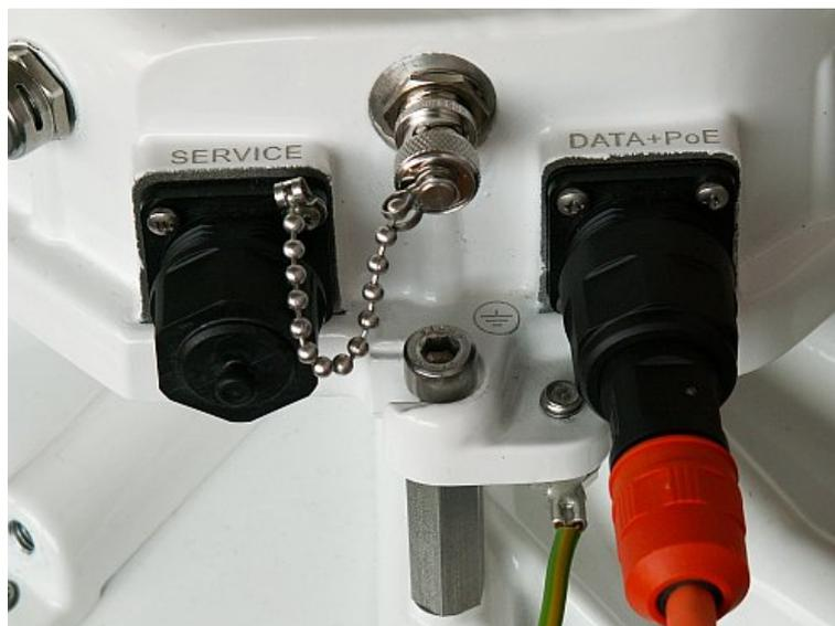
Fig. 3.3: RAY microwave bridge – connectors
