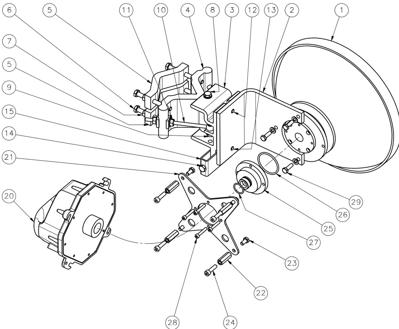
Fig. 5.20: Installation diagram for the Arkivator antenna, 30 and 60 cm
