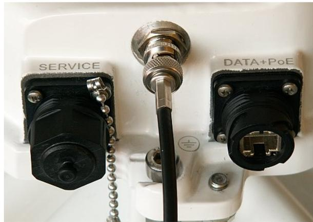
Fig. 5.68: Connecting a voltmeter to the BNC connector.
