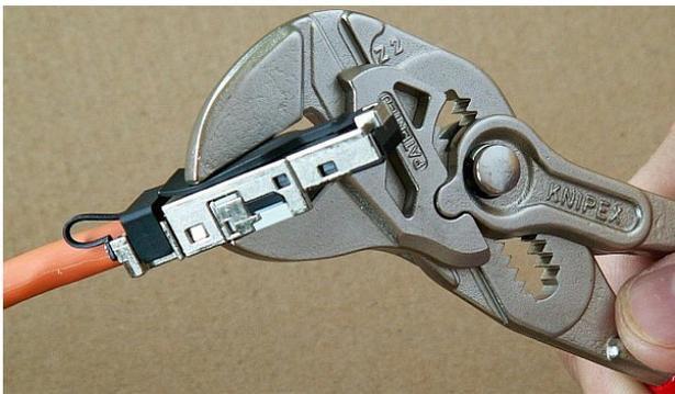
Fig. 5.58: Clamping the internal connector together with pliers
