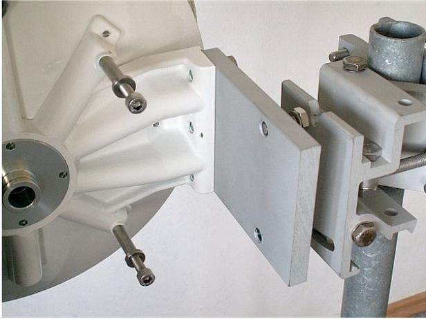
Tighten both bolts to the plate before continuing with installation to prevent any unnecessary movements of the whole equipment. Before precisely adjusting the vertical direction of the antenna upon completing installation it will be necessary to unscrew them again as the lower bolt passes through the adjustment block and the upper one serves as the axis of rotation.
