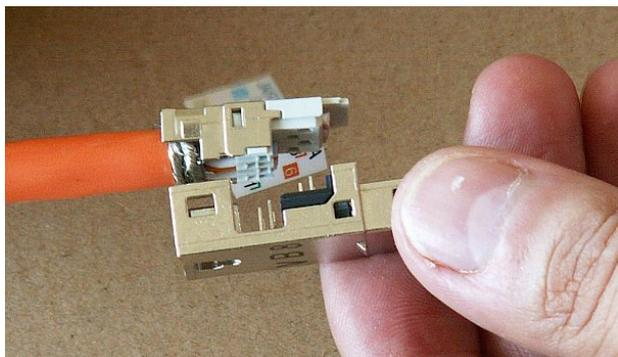
Then slide the protective cover onto the connector. It must fit into the grooves after snapping into place. Finally tighten the nut on the cover to seal the point where the cable enters the connector.
