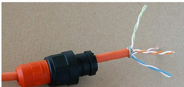
Fig. 5.36: Separated pairs of conductors
