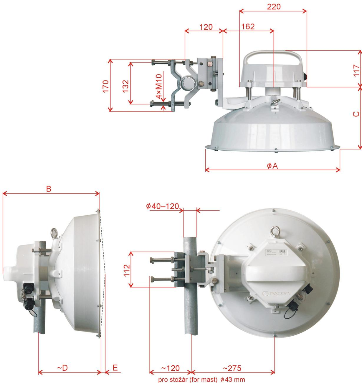
Fig. A.1: Dimensional layout of the RAY10 with the Jirous antenna
