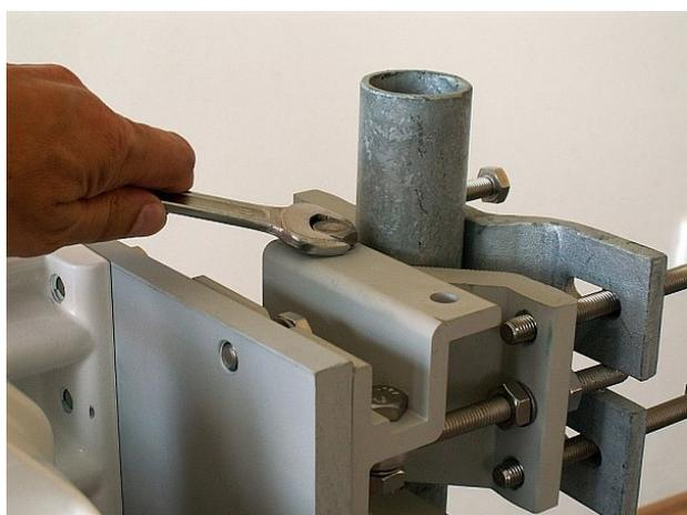
Fig. 5.19: Tightening the axis at the bracket
