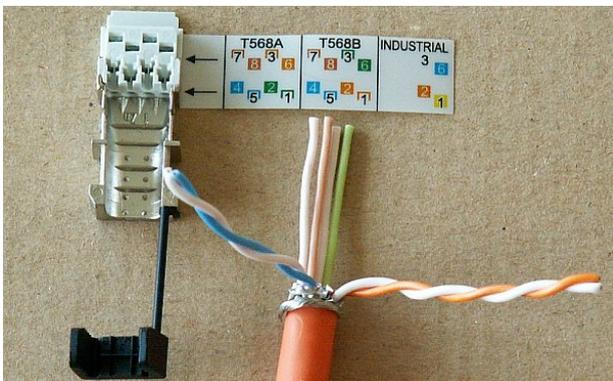
Fig. 5.52: Lower two pairs ready for inserting
