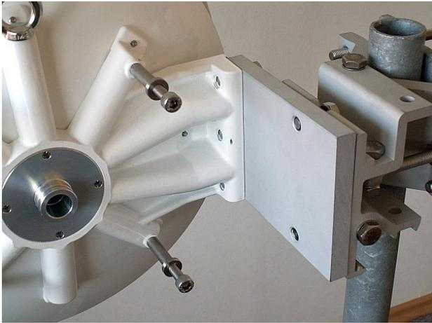
Fig. 5.11: Correct position of the mounting plate
