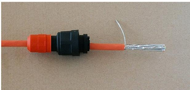
Separate individual pairs of conductors, remove the aluminium shielding from them, cut it off, and
