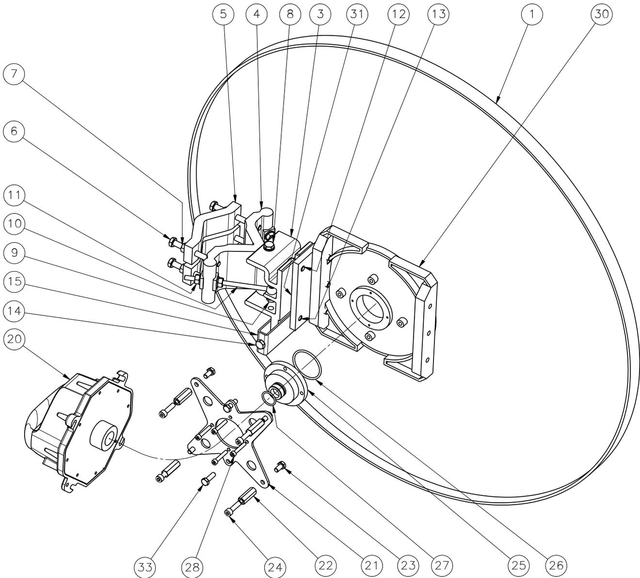
Fig. 5.21: Installation diagram for the Arkivator antenna, 99 cm
