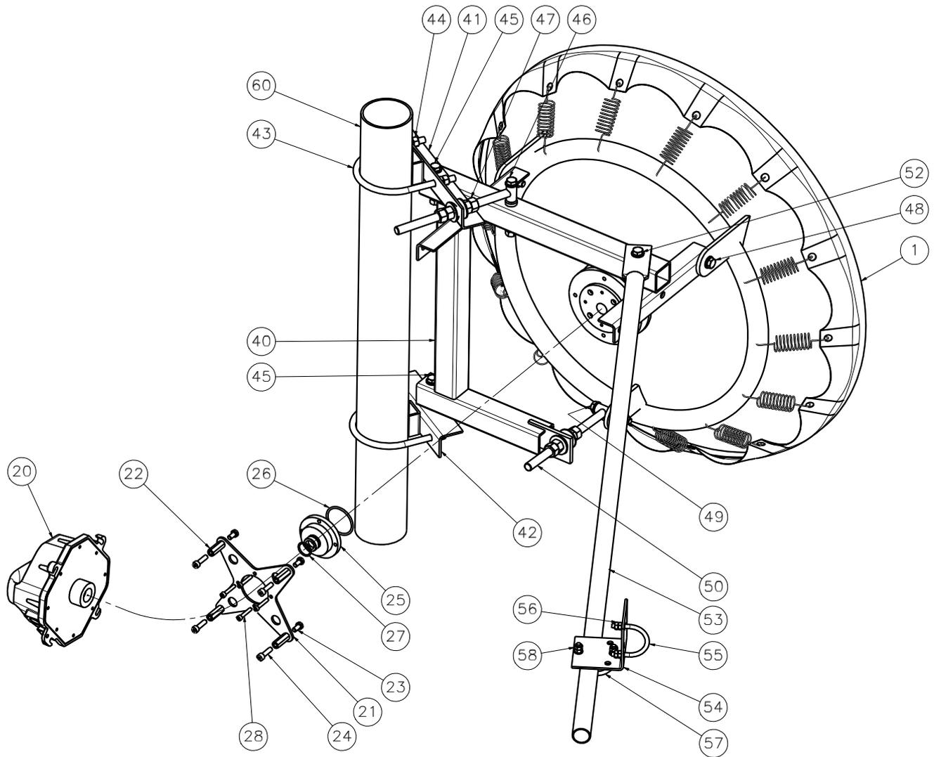
Fig. 5.25: Installation diagram for the Arkivator antenna, 120 cm
