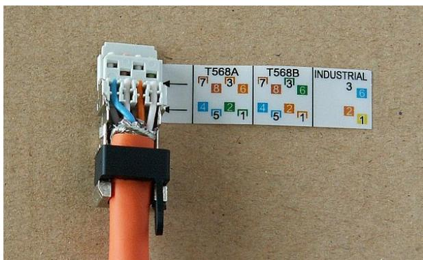
Fig. 5.56: Inserted and trimmed conductors
