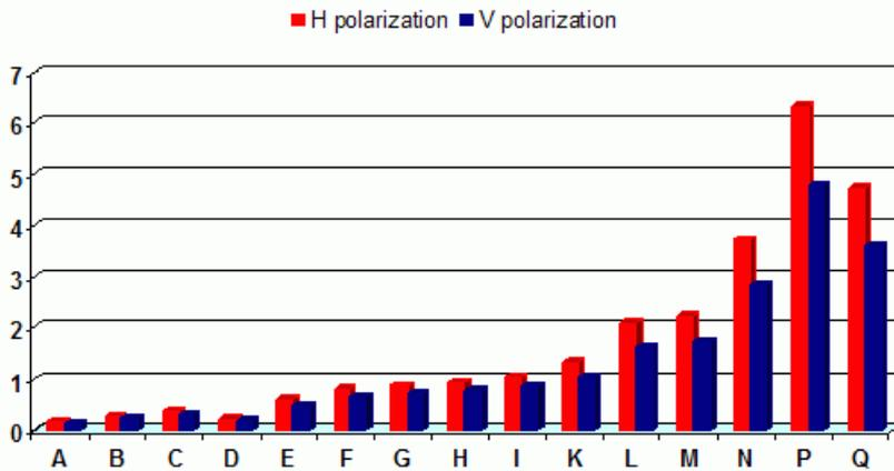
Fig. 2.2: Specific rain attenuation  $\gamma_{R_{0.01}}$  (dB/km) for H, V polarization and rain zones at 10 GHz
