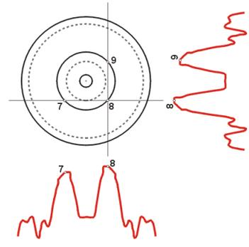
Fig. 5.71: Radiation diagram – incorrect adjustment
