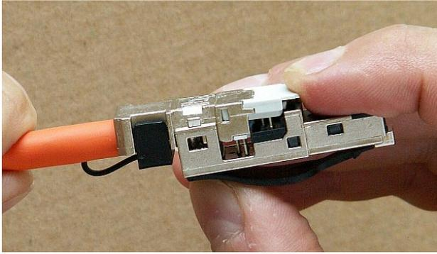
Fig. 5.57: Fitting the mate to the internal connector
