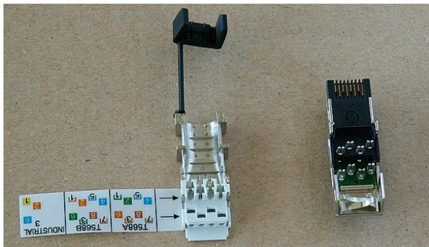
Fig. 5.45: IE-PS-RJ45-FH-BK connector before fitting
