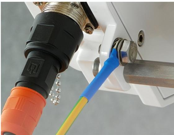
Fig. 5.65: Protective conductor at the FOD unit
