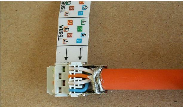
Fig. 5.40: All conductors in the connector
