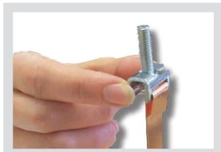
1. Pull the copper tape through the insert and bend
