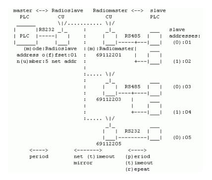
The Slave PLCs are connected individually or in groups to the MORSE CU (communication unit, modem, radio), which locally take on the function of the Master PLC.
