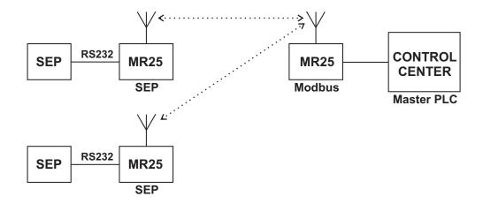
3. Connection of 1-3 SEPs over an RS 232 link to a common MR25 with control center. Functions as in example 2.
