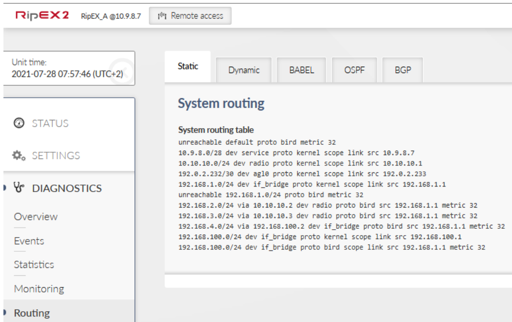
Fig. 6.17: RipEX_A – System routing
