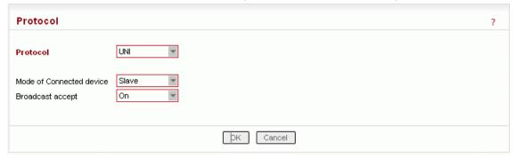
If the SCADA device connected responds to the message within a timeout of 500 ms, the source IP address of the received UDP datagram is used as the destination for the response.(Note only one packet is accepted as a response). When the timeout expires, all messages received by the serial interface are discarded.
