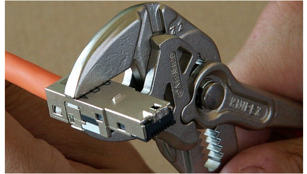
Fig. 5.44: Squeezing the connector until the locks snap into place
