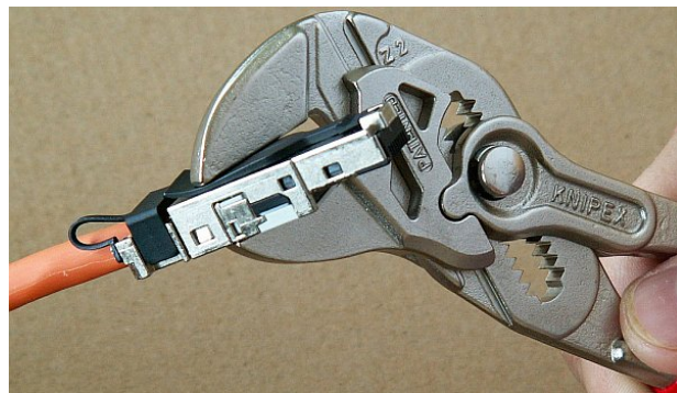
Fig. 5.60: Clamping the internal connector together with pliers
