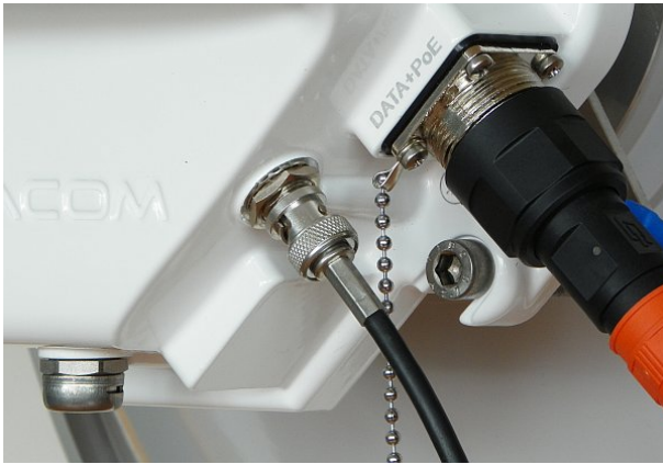
Fig. 5.70: Connecting a voltmeter to the BNC connector.
