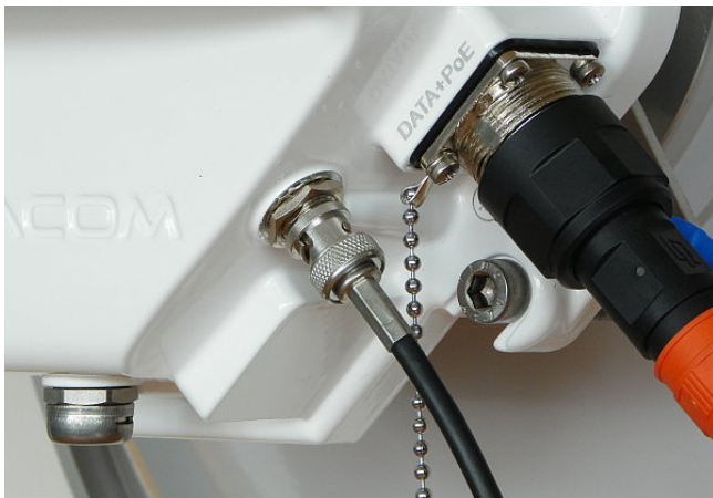
Fig. 5.29: Connecting the FOD communication unit
