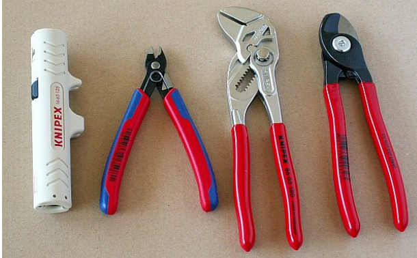
Fig. 5.31: Tools for fitting connectors
