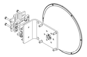
Fig. 2 Antenna with massive bracket (back side)
