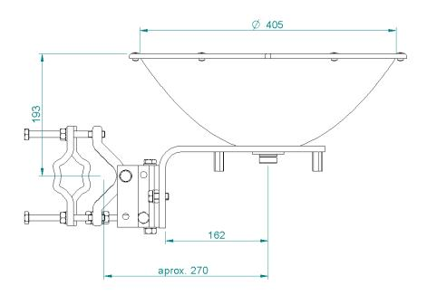
Fig. 1 Antenna dimensions
