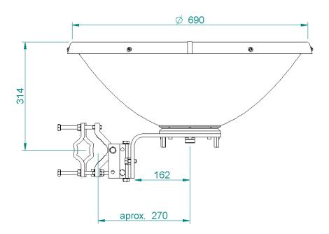
Fig. 1 Antenna dimensions
