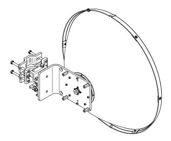
Fig. 2 Antenna with massive bracket (back side)
