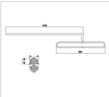
The offset antenna OV138.1 is a base antenna for radiostations working in bands of 135-152 MHz. This antenna has a slightly directional radiation pattern with the gain of 2.5 dBd. The antenna is broadband and that is why it is suitable for duplex operations.
