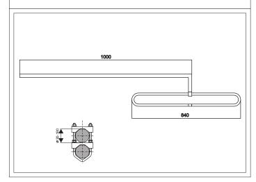
The offset antenna OV160.1 is a base antenna for radiostations working in bands of 150-174 MHz. This antenna has a slightly directional radiation pattern with the gain of 2.5 dBd. The antenna is broadband and that is why it is suitable for duplex operations.
