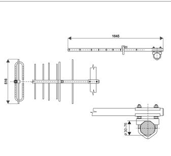
The antenna SA300.9 is designed for base radiostations working in bands of 300-355 MHz. It can be used for receiving and transmitting till 200 W. The antenna has a directional radiation pattern, is broadband and that is why it is suitable for duplex operations.
