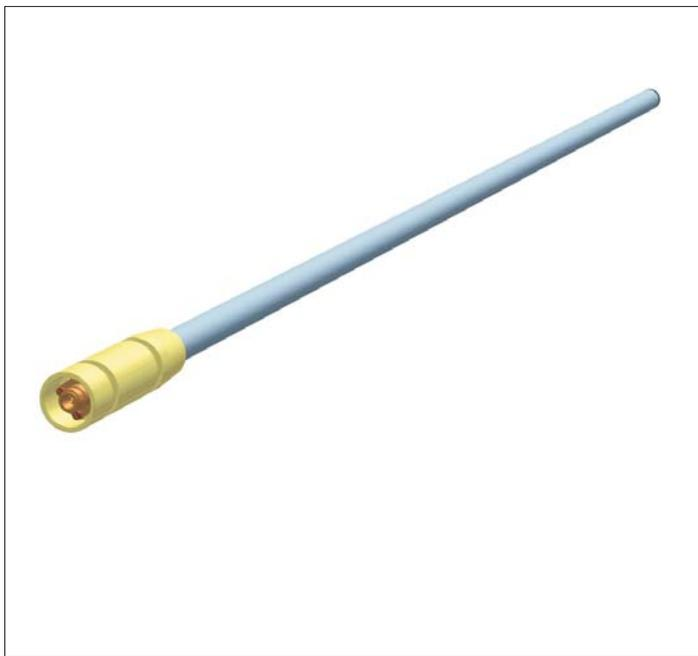
The omnidirectional antenna KA330.3 is designed for base radiostations working in bands of 330-355 MHz. The antenna has a omnidirectional radiation pattern with the gain of 3 dBd and is suitable for the top-mounting. The antenna is broadband and that is why it is suitable for duplex operations.
