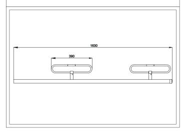
The offset antenna OV350.2 is a base antenna for radiostations working in bands of 350-380 MHz. This antenna has a slightly directional radiation pattern with the gain of 6.7-7.4 dBd. The antenna is broadband and that is why it is suitable for duplex operations.
