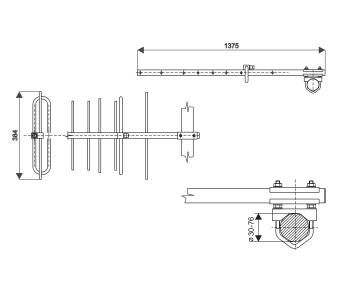
The antenna SA380.9 is designed for base radiostations working in bands of 380-410 MHz. It can be used for receiving and transmitting till 200 W. The antenna has a directional radiation pattern, is broadband and that is why it is suitable for duplex operations.
