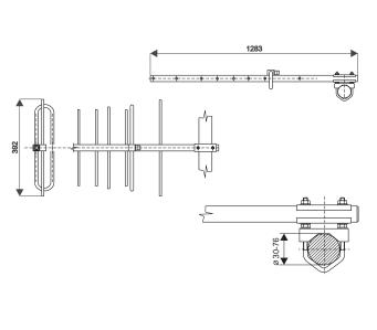
The antenna SA400.9R is designed for base radiostations working in bands of 400-435 Mhz. It can be used for receiving and transmitting till 200 W. The antenna has a directional radiation pattern, is broadband and that is why it is suitable for duplex operations.
