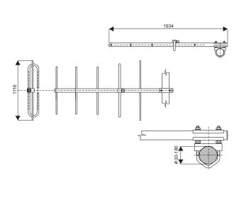
The antenna SA138.5 is designed for base radiostations working in bands of 136-146 MHz. It can be used for receiving and transmitting till 200 W. The antenna has a directional radiation pattern, is broadband and that is why it is suitable for duplex operations.
