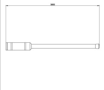
The omnidirectional antenna KA140.3 is designed for base radiostations working in bands of 146-158 MHz. The antenna has a omni-directional radiation pattern with the gain of 3 dBd and is suitable for the top-mounting. The antenna is broadband and that is why it is suitable for duplex operations.
