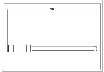
The omnidirectional antenna KA300.3 is designed for base radiostations working in bands of 300-330 MHz. The antenna has a omnidirectional radiation pattern with the gain of 3 dBd and is suitable for the top-mounting. The antenna is broadband and that is why it is suitable for duplex operations.
