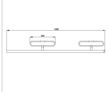
The offset antenna OV400.2R is a base antenna for radiostations working in bands of 400-435 MHz. This antenna has a slightly directional radiation pattern with the gain of 6.7-7.4 dBd. The antenna is broadband and that is why it is suitable for duplex operations.
