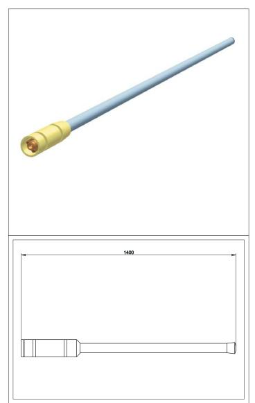
The omnidirectional antenna KA400.3 is designed for base radiostations working in bands of 440-470 MHz. The antenna has a omnidirectional radiation pattern with the gain of 3 dBd and is suitable for the top-mounting. The antenna is broadband and that is why it is suitable for duplex operations.
