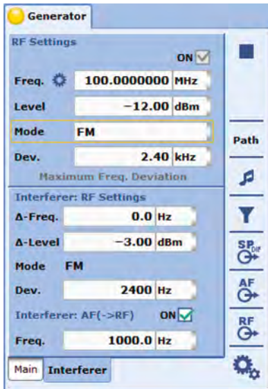
Frequency modulation with an integrated interfering signal.
