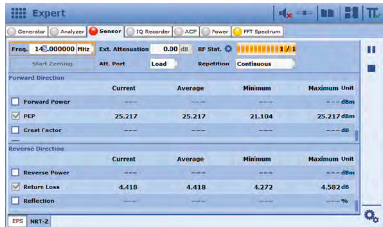
Measurements with R&S®NRT power sensor connected to the R&S®CMA180.
