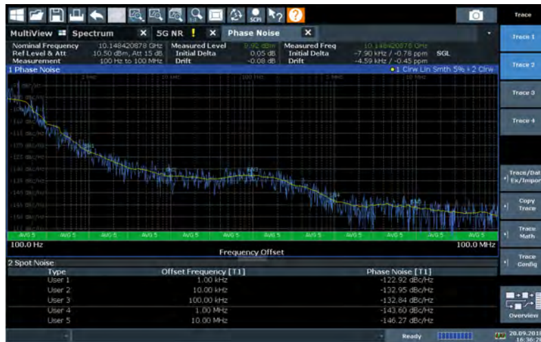
Phase noise at 10 kHz offset from a 10 GHz carrier: typical -133 dBc (1 Hz)
