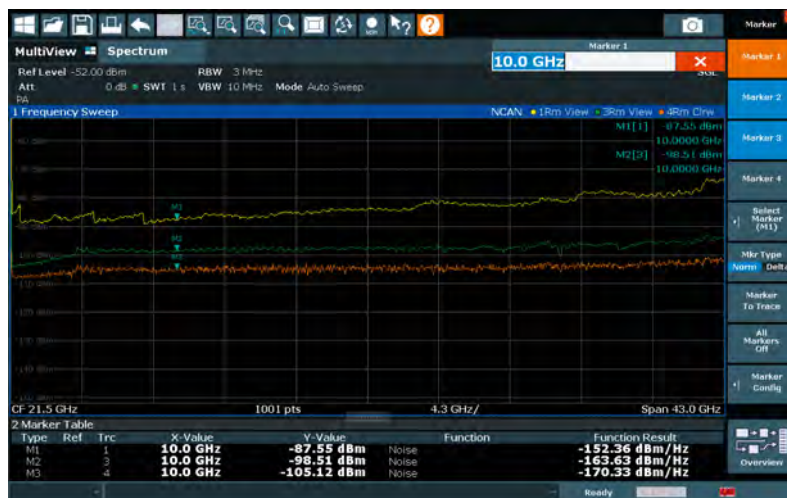
Displayed average noise level (DANL) of an R&S®FSW43 with preamplifier and noise cancellation switched on/off
